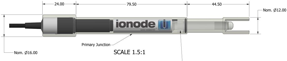
**Temp. Range:** 0-60<sup>°</sup>C **Body Material:** Polypropylene Reference Potential: -44mV vs SCE **Junction:** Sleeve Junction Max. Pressure Rating: 40 PSI Submersible: Yes
